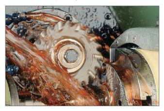
Heat Forged Steel Bodies for Large Diameter Bits. No router bits are exactly the same, sometimes not even in the way they are made. Certain bits require a few more steps than others, like heat forging the steel of larger diameter bits before turning it down into precise bit bodies. This extra step produces a radial grain orientation which gives large diameter bits extra strength and durability.
