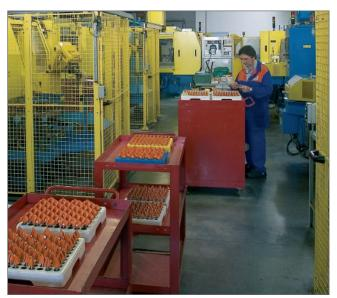
Loading the automated multi-axis CNC sharpening machines.
