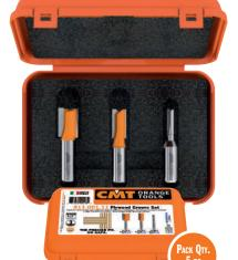
These groove bits are specifically designed to rout grooves and dadoes for joints in plywood. This means they match the true thickness of the material, producing tight, accurate joints. Use our 23/32" bit for 3/4" plywood, 31/64" bit for 1/2" plywood and our 15/64" bit for 1/4" plywood. No gaps. No sloppy joints. No worries! These money-saving 3-bit sets are available with 1/2" or 1/4" shanks.
