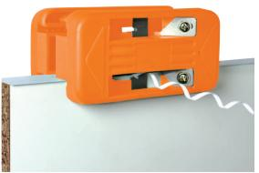
Attach this trimmer to your workpiece, press both ends against the board for a cutting range between 13mm (1/2") and 25mm (1"), move the trimmer in the correct direction indicated by the arrow. This will cut on both sides easily. The first cutter will cut straight, the second one can be adjusted for a tapering cut. Both cutters are made from high-quality hardened steel and can be easily replaced when worn out.
