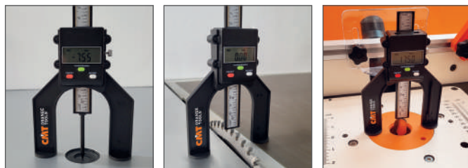
Place your gauge on a flat surface and set to zero
