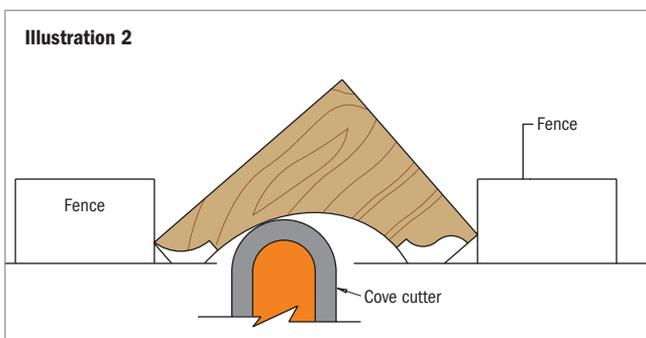
top. Turn on the power and feed the stock slowly between the fences; after each pass raise the cutterhead another 1/16". Remember to use a guard and push blocks for added safety.
