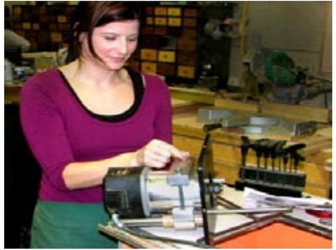
The round body of the router fits into the lift's cradle and is quickly locked in place.
