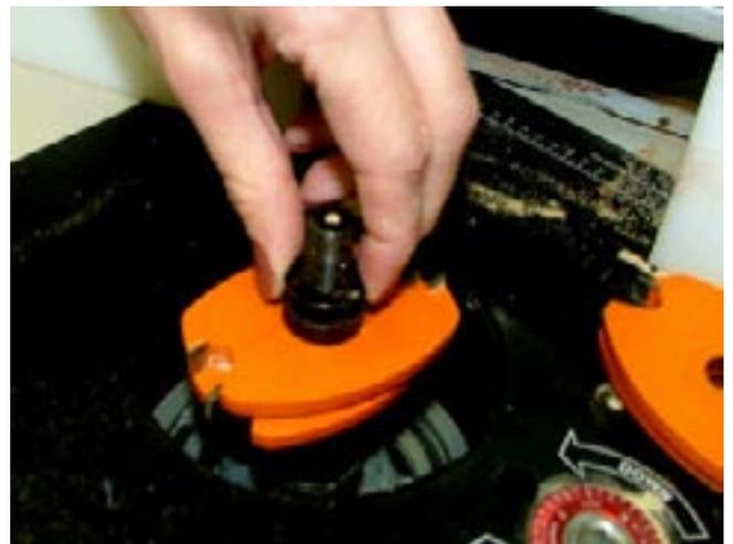
The adjustment works. She has a tenon that is just the right thickness. Now, she can make wider mortises or use a hand saw to trim the tenon width. The hard part is done. The tenon fits well and she now can record the combination of spacers that will allow her to replicate the 5mm tenon at any time.
