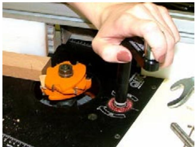
Just as she would when cutting a coped end of a rail, Andrea runs the sample through the cutter using a square scrap of MDF to serve as a backer board and help her keep the sample square to the fence.
