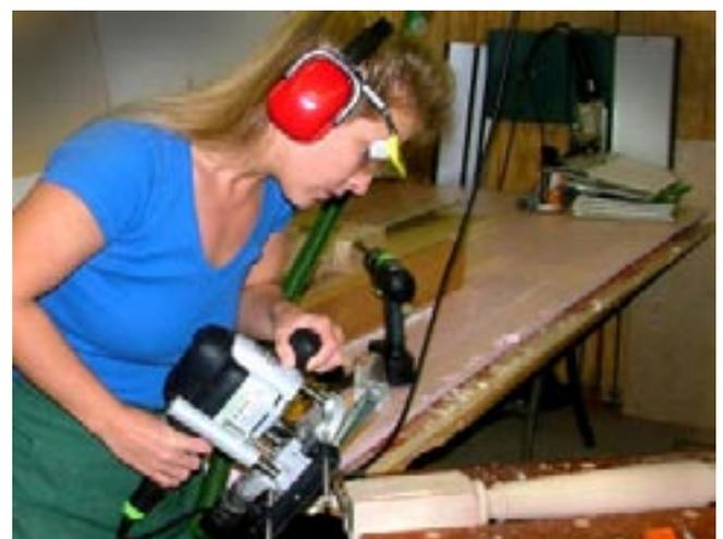
The CMT Tenon Cutter set makes matching the tenon width to the mortise a relatively easy task. It is just a matter of removing or adding a combination of spacers.
