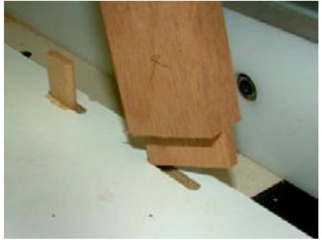
Andrea is proud of her new found skill. The CMT Tenon Cutter is a precision tool that allows precision cuts. It can produce tenons with thicknesses between the 3/16" and 3/8" shown above – and in metric as well.
