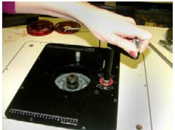
This is the product shot from Woodpeckers website. I show it because it displays the other way to adjust the height of the router. The steel L-handle device is inserted and then turned 1/4 turn to allow the router to be brought up or down quickly. It is a nice picture isn't it?
