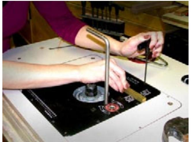
She takes a few minutes to adjust the insert height so that the top is in perfect alignment with the router table top.
