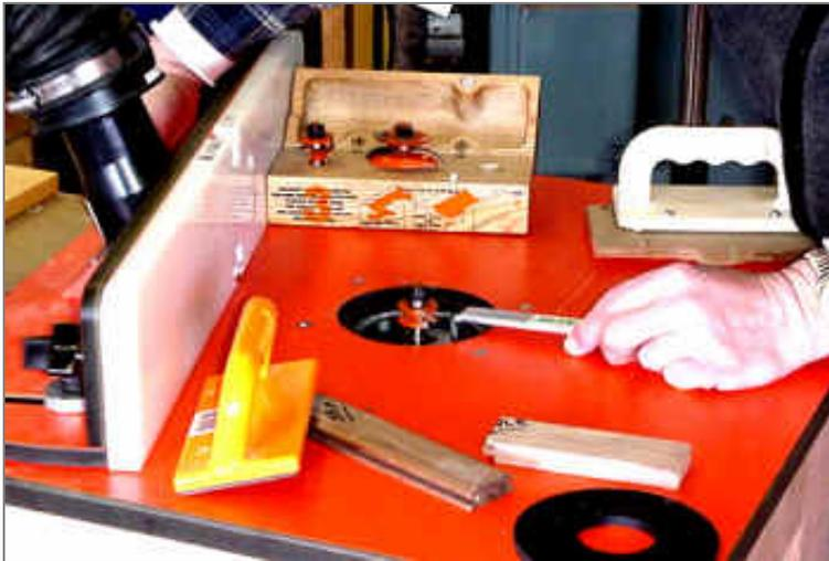
I use the sample piece to double-check the height. When the router bit is rotated, the cutter should just "kiss" the groove of the sample. It does.
