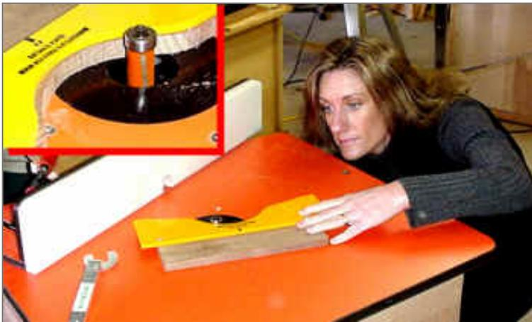
**She has installed a trim bit so that the bearing is in contact with the template and the cutter covers the wood. The inset shows a closer, "birdseye" view.**
