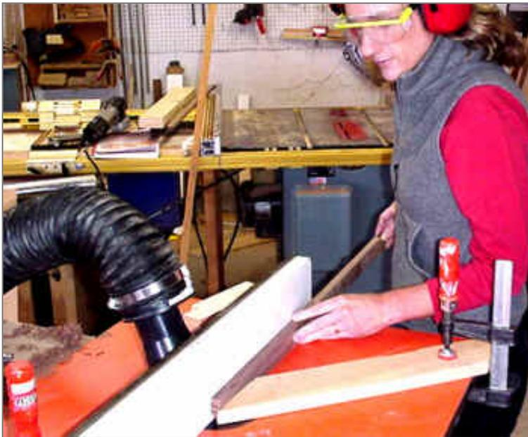
**It is funny how coming back to a problem another day can make the problem go away. I used a classic bit on the base piece that is now installed. The piece I am now marking was cut with another ogee cutter using only a portion of the profile.**
