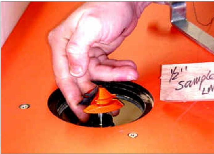
**I have installed the locking miter bit. I have also brought out my sample that I cut from the same stock. I will use that to setup the router bit height and fence depth.**
