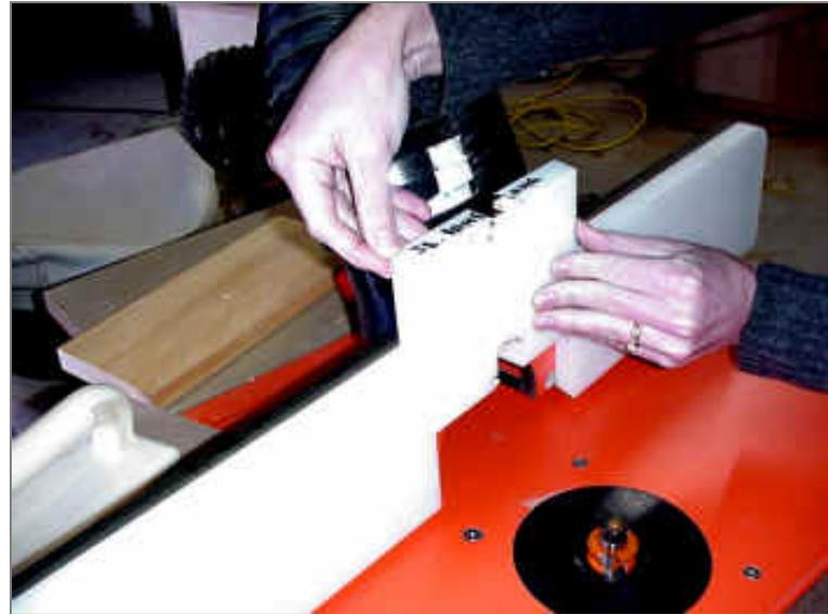
**She brings the fence forward until it is aligned with the pattern bearing and locks it in place.**
