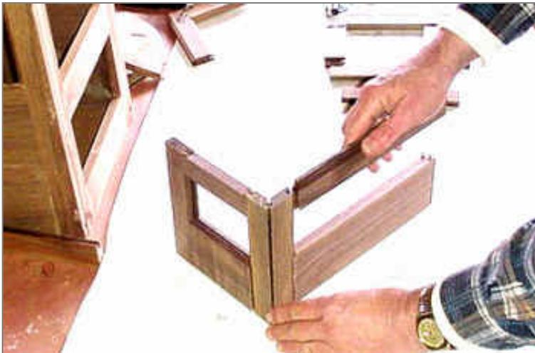
**I am only dry fitting at this point and want to give you an idea of how the sections go together. The locking miter joint, we did first, will be the corner post. [Note, the gap at the corner is because I am not holding the corner together.]**
