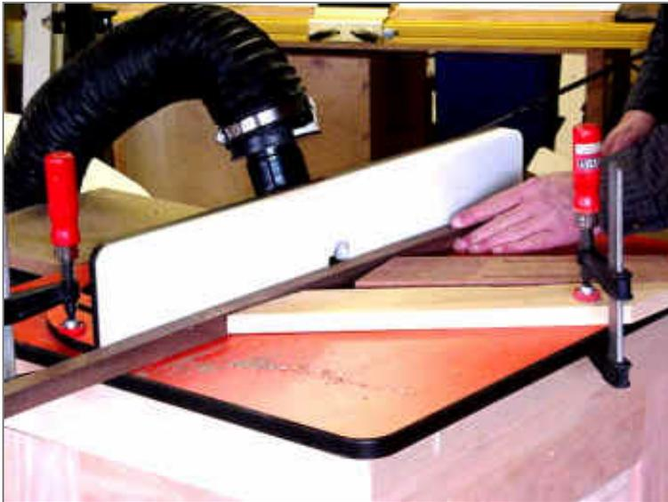
At the router, I make several passes with the rabbeting bit. This piece will be an outside corner molding so I want to rabbet the inside to leave 1/4" sides. The two finger boards help to keep the stock square against the fence.
