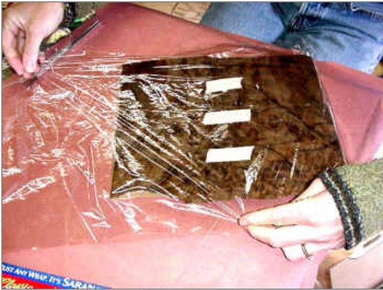
**Beth uses Saranwrap to cover the top and bottom. This keeps any glue that is squeezed out from attaching to the outer clamping boards.**
