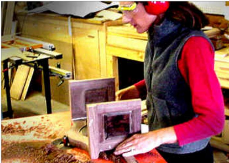
Beth is doing the final trimming of the molding that she applied to the top section. If you recall, the bottom was shaped using one of the templates, but the piece was too small to shape the top edge at that time. It is easy to do after it has been attached to the piece.
