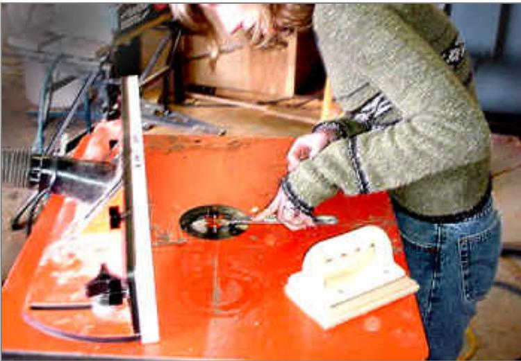
Having placed the sample on the infeed side, Beth has installed two feather boards. One is clamped to the fence and holds the piece down on the table. She is clamping the second to the table having positioned it to hold the piece tight against the fence.
