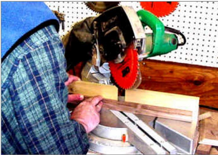
When we started this project, I reported that I installed a brand new CMT compound miter saw blade. It has performed flawlessly in all the cross cuts so far. Now, it is making picture frame perfect corner cuts. [By the way, I have retracted the guard only for the picture. It releases as soon as I start the cut. Table saw guards should be so well engineered.]]
