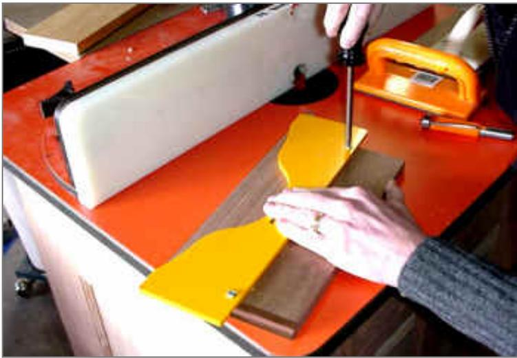
**With the ends of the rails coped, Beth attaches one of the templates to a rail piece which will be shaped with the graceful crown at the top of the clock.**
