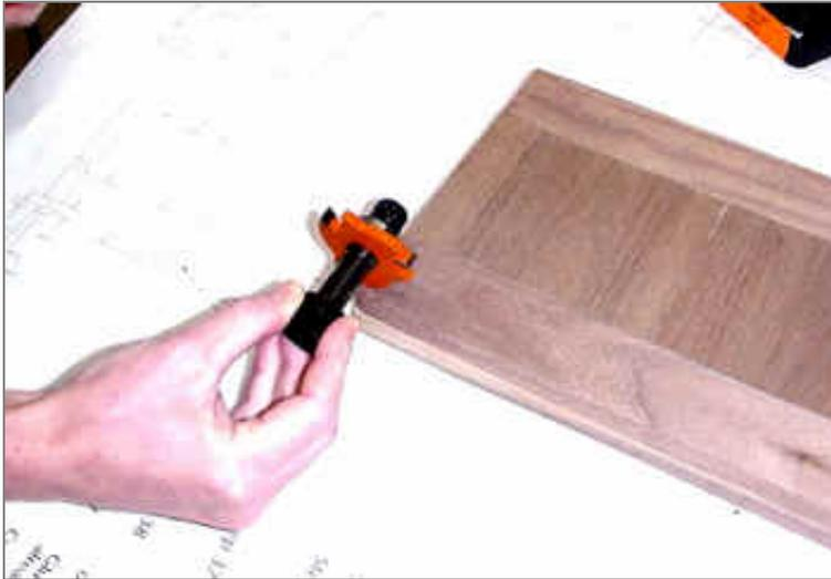
Two grooves will be cut into the length of both sides. The tongue is designed to cut a 1/4" width. The bearing allows a 3/8" depth of cut much too much for 1/2" stock. The plans explain how to swap the pattern bearing to make a 1/4" cut. Rather than to change bearings, Beth and I decide that we can use the fence to limit this depth.
