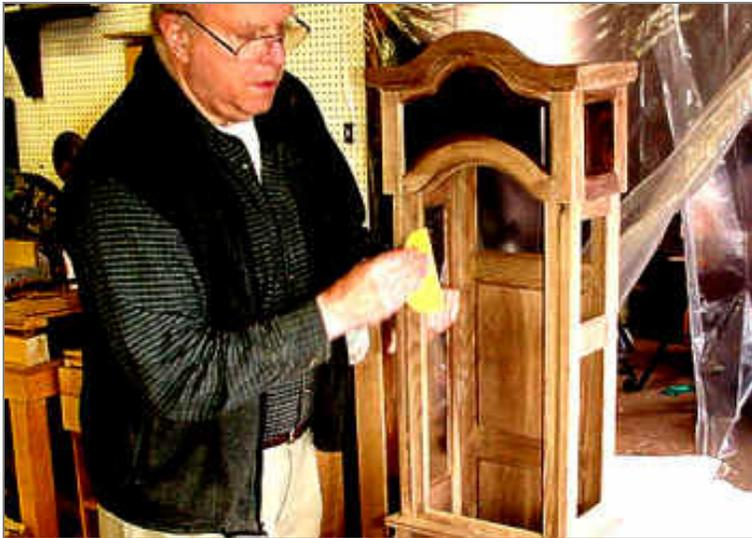
**This is a good time to sand of few of the edges that haven't yet been touched. I am "feathering" the edges of the door recess.**
