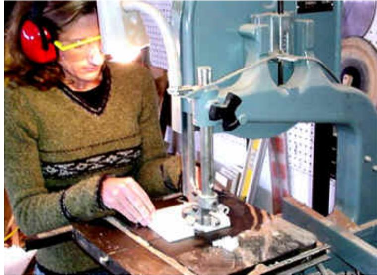
With the fence insert cut, she starts the cutting of the panels by making shallow cuts and then moving the fence back until the bearing is aligned with the fence.
