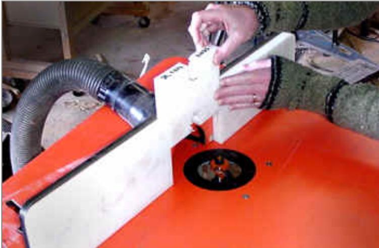
She installs the fence insert that has been cut for this bit.
