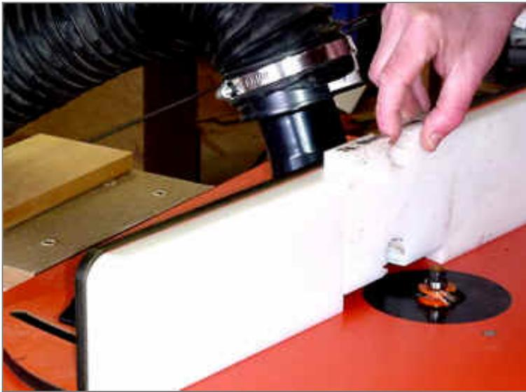
**The correct fence insert is installed. Since I have cut this insert in the other edge of the same insert, all I have to do is switch it end for end.**
