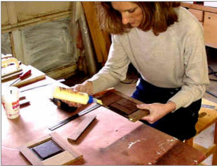
We found that there is a "best" way to add glue after dry fitting the assembly. She does not disassemble the entire frame, but instead, she removes one of the stiles at a time. With one stile off, she adds a touch of glue to where the rails will join the stiles.
