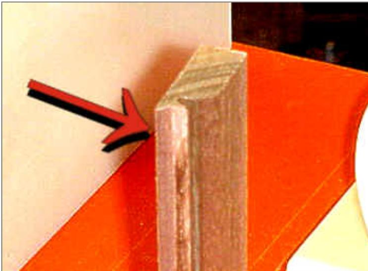
**This is the cut. The arrow points to the outside edge which should be knife sharp. If there is any width to it, the fence needs to be backed off slightly.**
