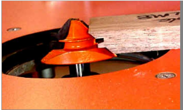
**Having a sample block does make the set up of any bit very fast and accurate. From this view, you can see that the bit height is not left to guess work or trail and error. It can be very exact.**
