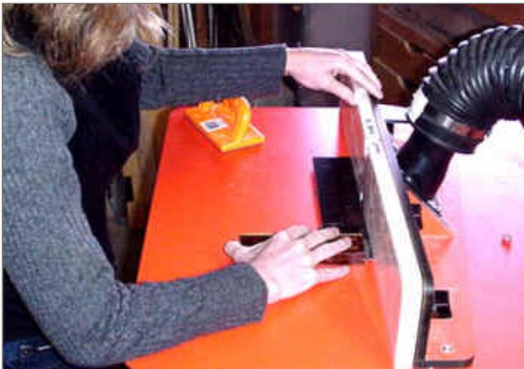
She makes the cut on the ends of each of the rails. Her right hand is holding the push pad that is attached to a piece of 1/2" MDF. This serves as a push stick and as a backer board. The push pad in her left hand is used to keep the piece flat on the table and against the fence.
