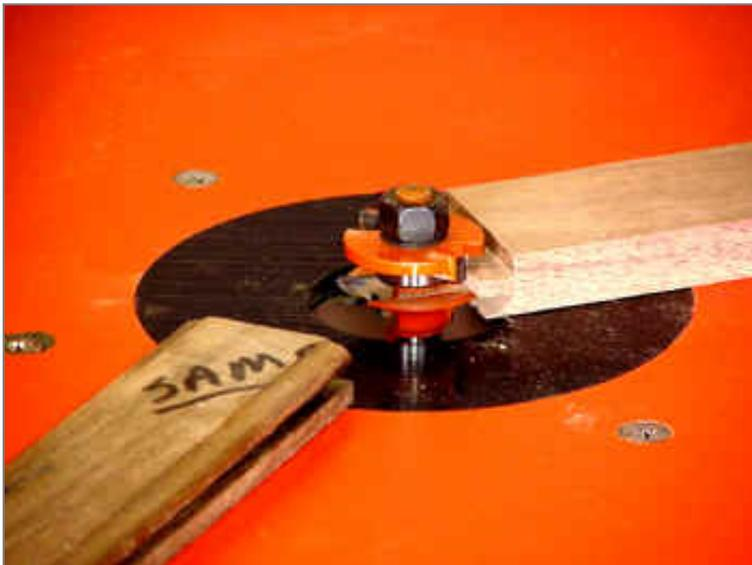
I have installed a throat plate and am now setting the router bit height using the coped end of my sample.
