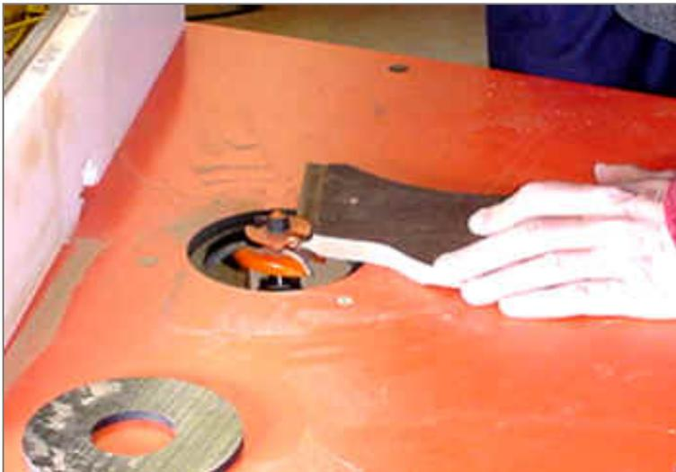
**With each of the panels at their right dimensions and shapes, I am ready to cut the raised panel profile.**
