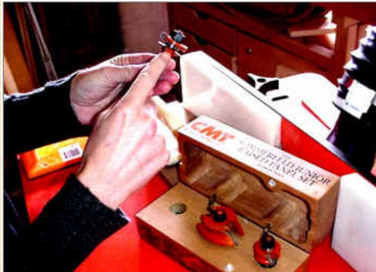
It is time to cut the cope ends on all the rails of the sides and the front panel. She selects the cope cutter it is the one with the bearing in the middle.
