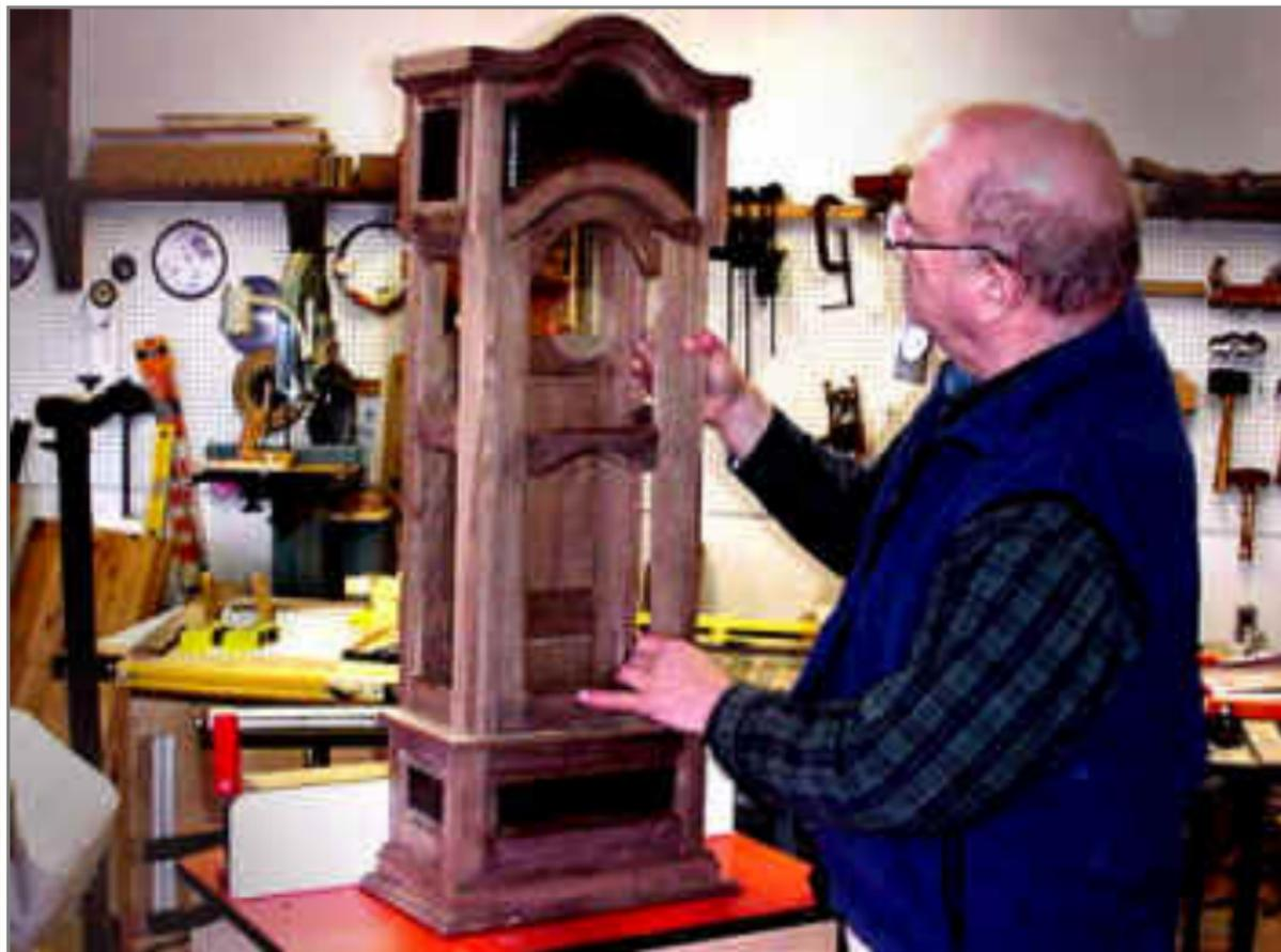
**I am holding the door in place. I have to find overlap hinges that will look right in this piece. Next, I have to mount the stage for the clock itself. Then we can move to the warmth (yea!) of the house for the finishing steps.**
