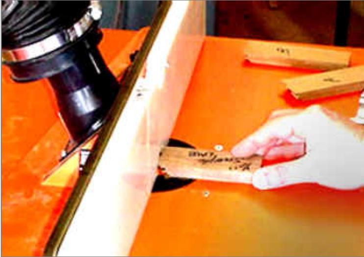
I will make one cut on each corner piece with the stock flat on the table. In my right hand I am holding the push block with the 1/2" MDF. This has the locking miter shape and is used as a backer board. I will push the stock through the bit with this hand.
