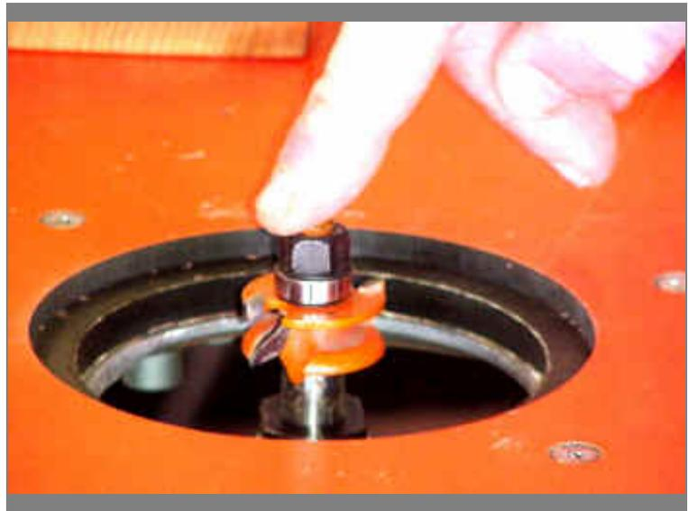
I tighten the bit using the bent wrench.
