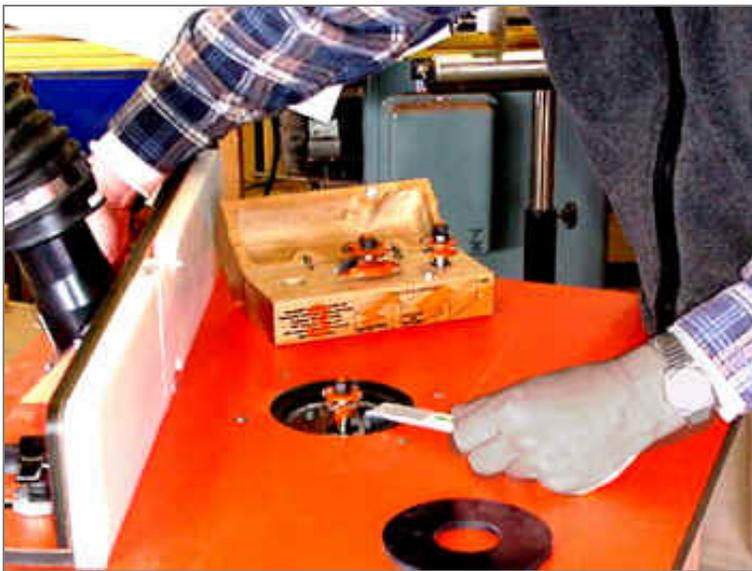
Using the bent wrench, I install the cope bit in the router. My right hand is holding the knob that is connected to the shaft lock of the Hitachi M12V router.
