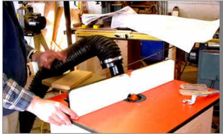
When the router comes to a complete stop, I move the fence into the bit and use the sample cut to adjust the fence depth.
