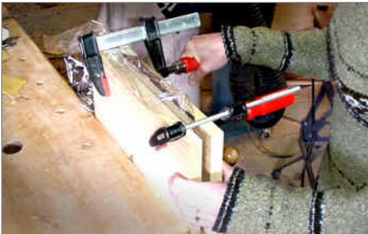
**She has clamped the sandwich in the bench vise and is adding a couple of hand clamps to further squeeze the package. She will leave it to set overnight.**
