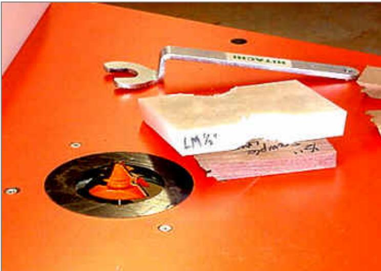
**I store the sample cut with the fence insert for that bit. This insert happens to have two profiles cut in it. One is for this bit in 1/2" stock and the other for 3/4" stock. Labeling helps to keep the inserts straight.**
