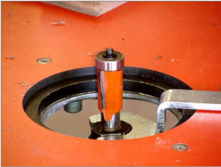
**I install my 1" pattern bearing bit. This close-up shows the "shear" angle of the cutter. This gives a smoother cut.**
