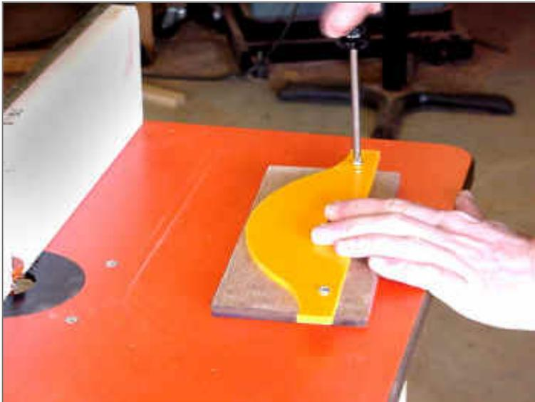
I, first, will attach the appropriate template to the dimensioned board. The instructions say to use two nails for this. I am using 5/8" sheet metal screws. I have pre-drilled the template to locate the screws well enough in so that the screw hole will not protrude in the raised panel cutter area. I am working from the back. The face is flat down on the table.
