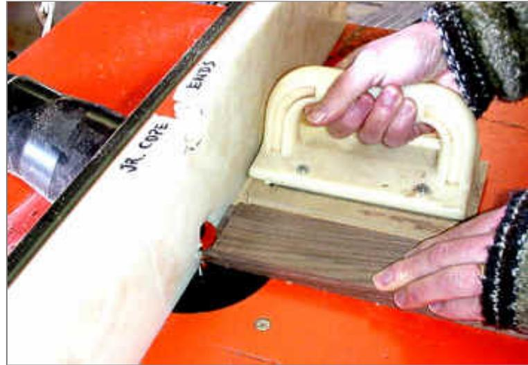
With the fence backed away and the insert removed, Beth changes the bit to the rail and stile profiling bit. Since it is a part of a matched set, the height should be right without any new adjustment. She checks it with the sample. It is. With this cutter's fence insert installed, she brings the fence up to the bearing, and she is ready to go.
