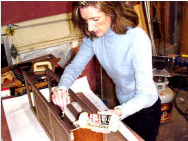
**Beth uses a brush to spread the carpenter's glue thoroughly over the tongue. There is a lot of gluing surface in this joint. It makes sense to use it.**
