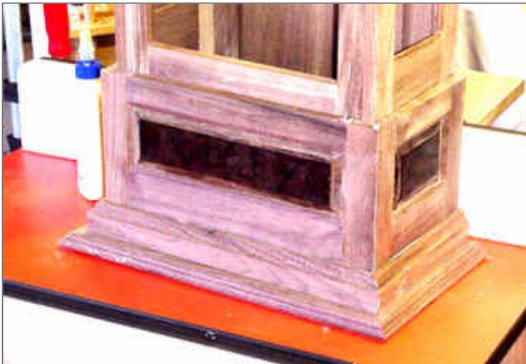
The two pieces of base molding are installed and look just fine. Now to attack the molding for just above the bottom raised panel frame. This is the one we were having trouble with yesterday.
