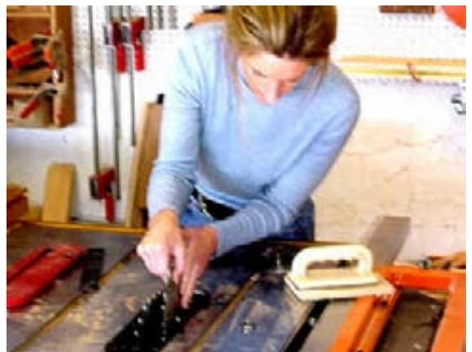
With the dado insert in place, she checks to see how smooth the small piece slides over the insert.
