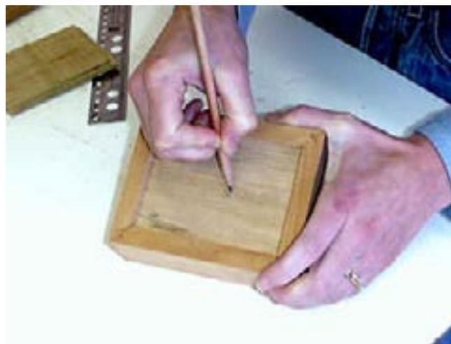
The clock requires a very exact  $1\frac{7}{8}$ " hole. It should be exact since the cases are friction fit in this hole.
