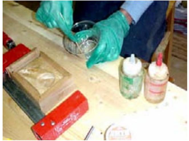
She uses a disposable “acid” brush to spread the epoxy over the locking miter surface.
