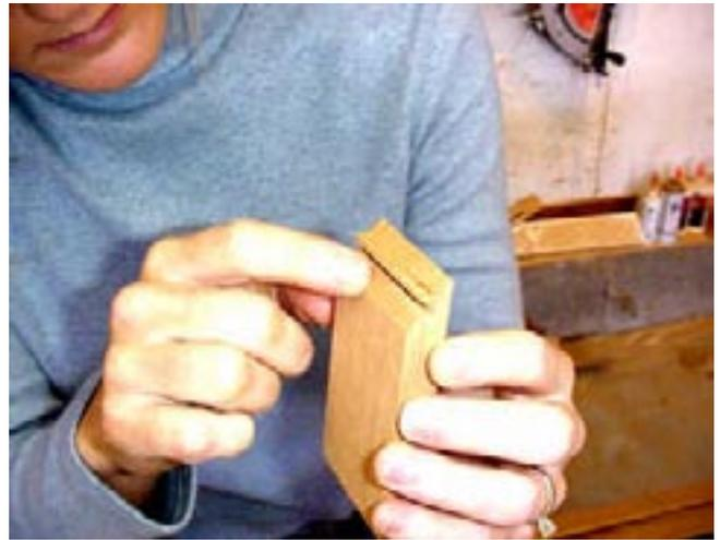
All the tops and bottoms are done. There are 20 pieces needed, and she did a few for spares. Each piece has two ends and each corner was cut in three passes. So there were a lot of cuts made to this stack, but in fact the whole process went smoothly and took about 12 minutes.
