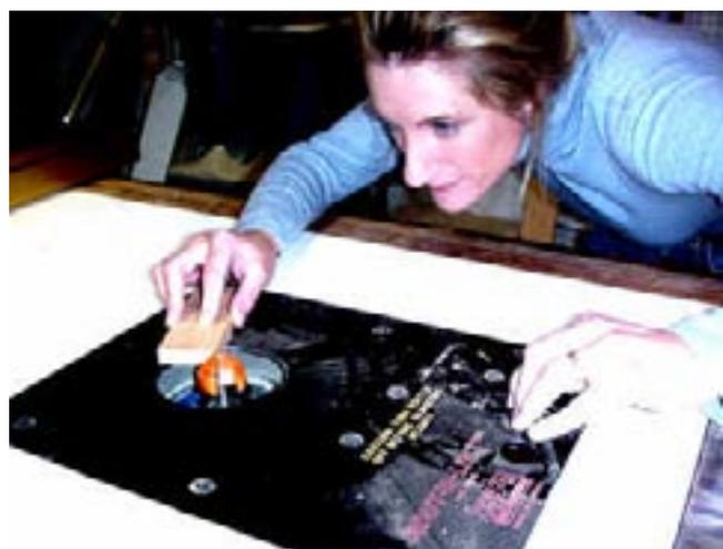
She marks the two sample pieces with an “A” and “B”. It takes just a few minutes to set the router height and fence accurately.
