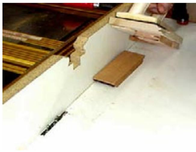
he makes the cuts. It took about 5 minutes to construct the special push pad, but it probably saved that much time, or more, in providing Beth a safer and quicker way to make the 80+ cuts,
