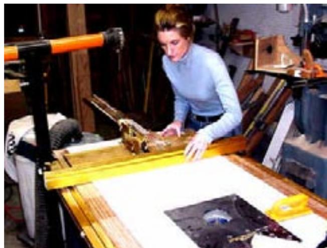
Holding the shaft lock knob in with her right hand, she uses the bent wrench to tighten the collet with the locking miter bit in place.
