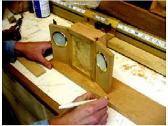
The new router table was all setup so Beth popped a new classic ogee bit into it and made the cut on three of the sides.
