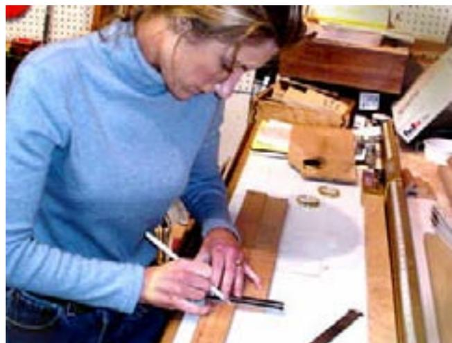
Since we want the grain to “wrap” around the box, Beth marks slant lines, or witness marks, so that the pieces can be re-oriented correctly after they are shaped.
