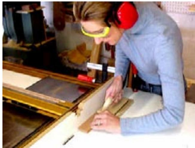
Here is the bottom of the MDF portion of the pushblock we used at the router. Beth has positioned the workpiece where it should be held.
