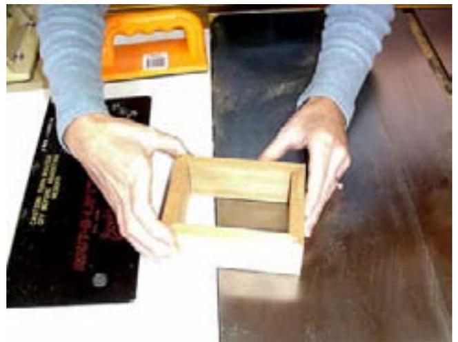
It's time to cut a groove for the front panel and a rabbet for the back.
