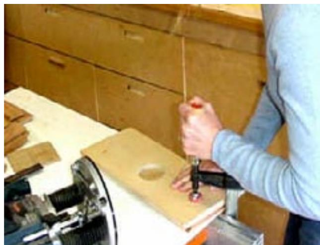
Beth makes a plunge cut using a  $\frac{1}{2}$ " up-spiral spiral bit and an edge guide that will give the  $1\frac{7}{8}$ " hole.
