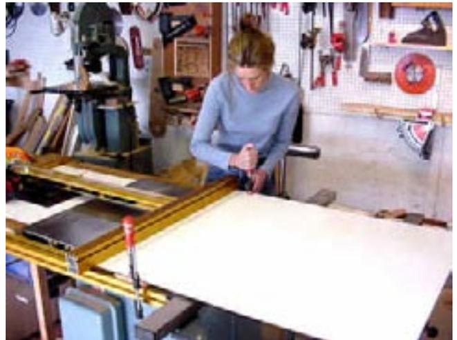
With the saw on, she slowly cranks the blade height adjustment until the blade cuts its own 'zero clearance' hole.
