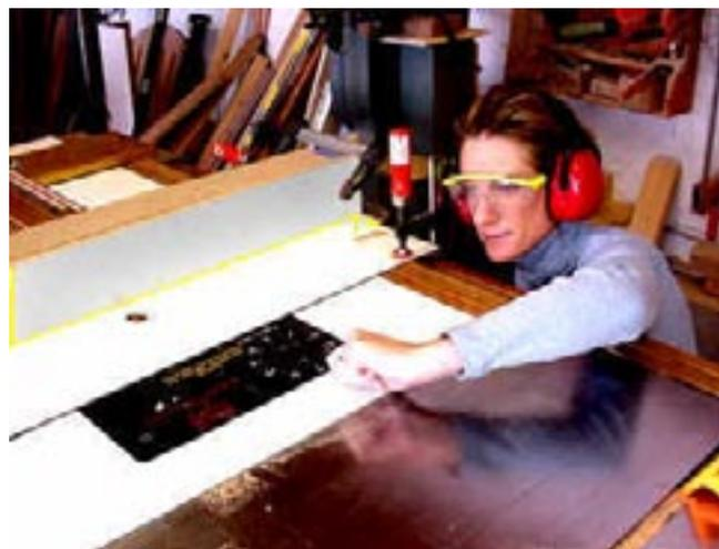
Then, she eases the fence into the spinning router to cut a fresh “zero clearance” hole for this setup.
