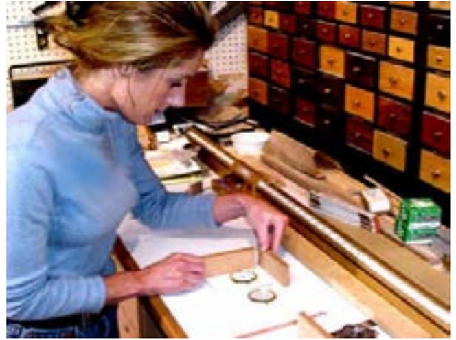
Well, we are getting somewhere. Here is what we are deciding: 1) have 1/2" margin around the clock face; 2) the width of the case will be 4" then; 3) 5" seems to be a nice, well proportioned height; and 4) this 4" X 5" box will set on a base that will raise it another 1/2". So that is our plan. We will set out to make boxes of this proportion.
