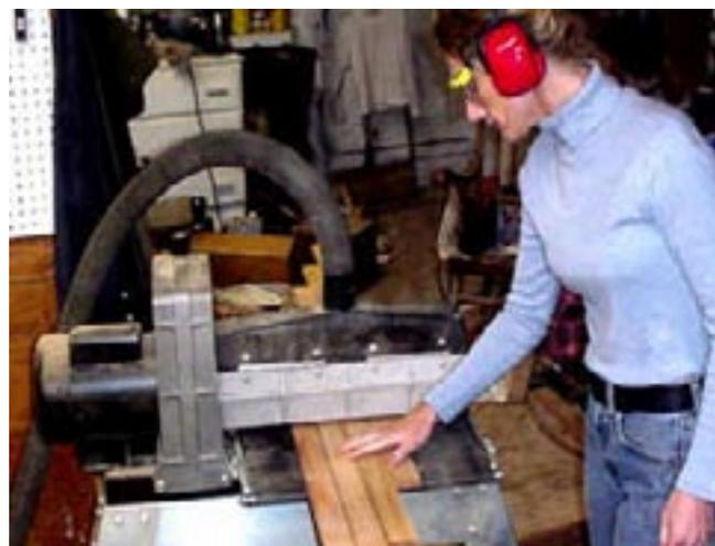
With the saw unplugged, Beth changes to the CMT 40-tooth, "General" blade. It is not thin kerf. While I enjoy using some of the thin kerf blades, I think the standard blade allows less flexing during cross cutting. I do use a single stabilizer on all blades.
