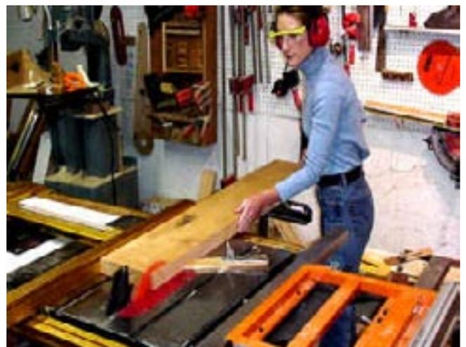
A few minutes later and Beth has the 5 strips we need for the clock cases. Keep in mind, that she moved the fence after each cut, using the blue 5/8" marks on the Incra TS-III template.
