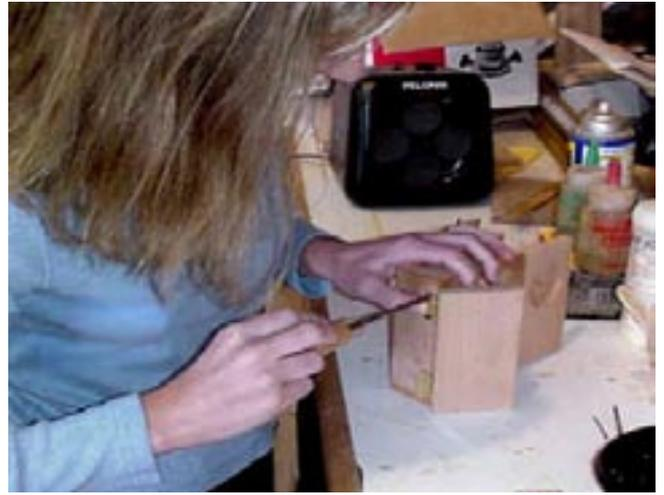
With the first box glued up, Beth tries mounting hinges. At this point, they are not mortised but just surface mounted. By the way, you can't see the center panel, since she has covered it with Saran wrap to protect the natural finish.
