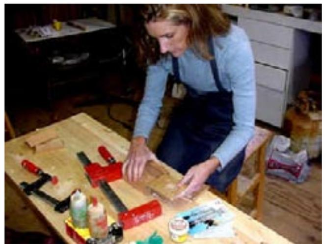
Beth mixes a very small batch of quick curing epoxy. This mix has about 6 minutes working time – just enough for assembling two clock cases.
