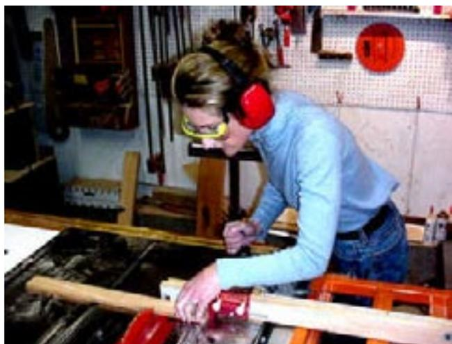
Since, each piece of stock will be cut 5”, then 4”, then 5” and another 4” to give the wrap around appearance, she uses a 1” spacer to make the 4” cut. Of course, if she were not worrying about the grain wrap-around, she could make all the 5” cuts and then the 4” cuts. Cutting in sequence takes a bit longer, but it will be worth it.
