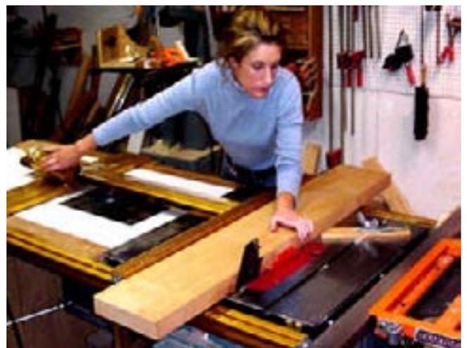
With the fence touching the cherry slab and locked, she moves the template for 5/8" spacing. This will give a 1/2" width board after the 1/8" kerf of the blade.
