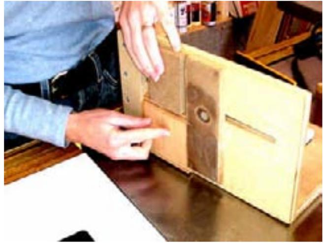
Now she makes the actual cuts. Her right hand keeps downward pressure on that piece of MDF, and her left hand keeps pressure on the jig. We have found that we can minimize tearout by keeping total control on the two small cherry pieces. Any movement on their part will cause a less than perfect cut.
