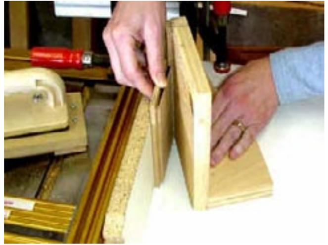
This is a better view of actually making the rabbet. The fence has been adjusted to allow a fraction less than 1/4" to be the width of the edge.
