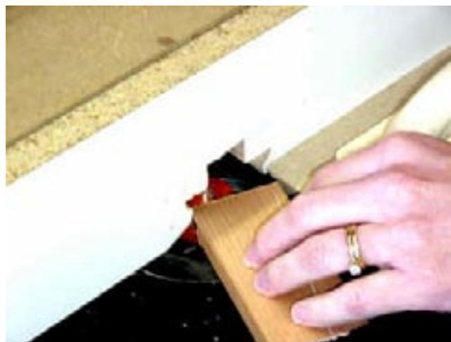
Rather than to cut a new board for the fence, Beth adds a thin sheet of white coated hardboard to the existing fence. I had bought a sheet of this inexpensive, plain white panel that is sold for use as bathroom tub surrounds. It is inexpensive (\$20 a 4' X 8' panel) and is useful for making templates and serves well here.
