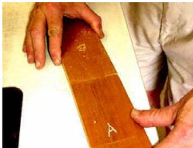
The first attempt is rarely right on, so I cut the first attempts off both boards, adjust the router bit height and re-do the test.
