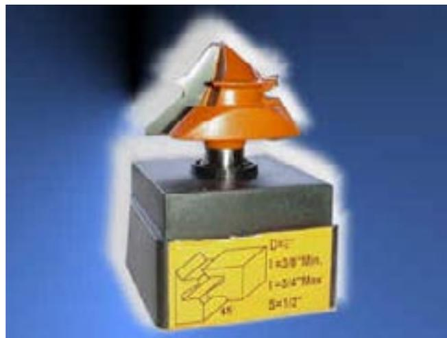
First, be sure to have a locking miter bit that can handle the stock thickness you want to join. In my case I am using CMT bits and the “baby locking miter” bit handles wood from 3/8” to 3/4”. The regular size locking miter bit is for thicknesses of 5/8” to 1 1/8”.
