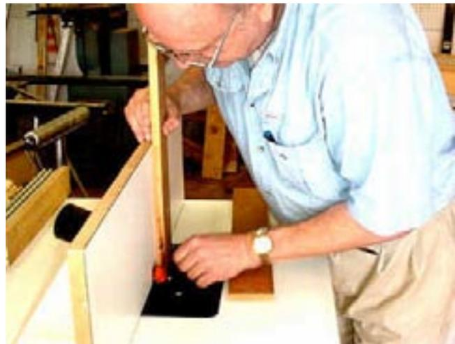
Here is what I am looking at. It is almost impossible to set the board to exactly where it should be...nor do you need to. Lock the fence to where you think the bit will cut the stock, and then use the "A" - "B" method to make the adjustments.
