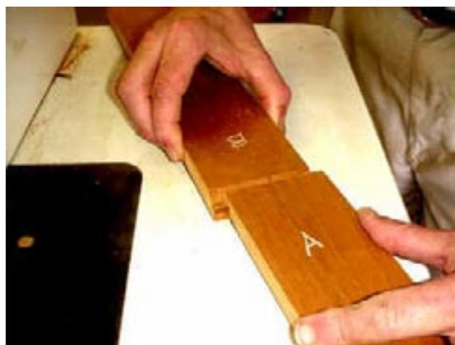
The resulting corner is as tight a 90o joint that you could ever want. What's more, you can make this joint on any thickness stock – within the range capability of your locking miter bit, of course.
