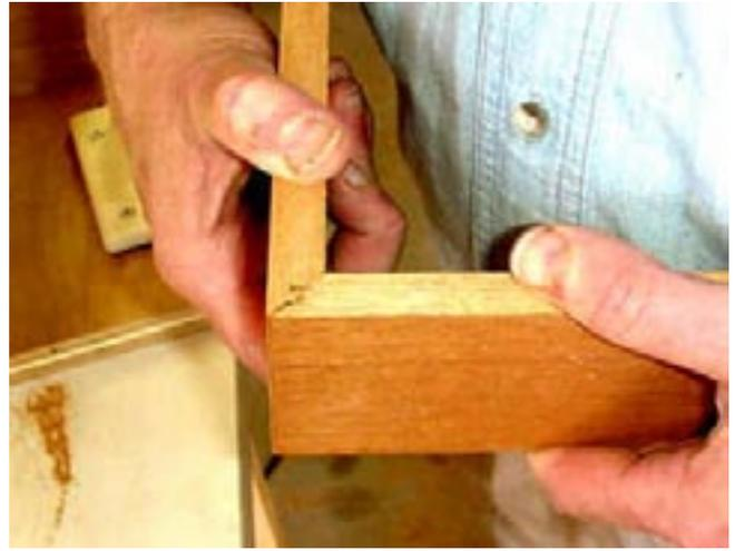
For this set up, I made three test cuts for the router bit height and another three for setting the fence. This photo shows how much stock I used to make these cuts (5” total). Not a bad price to pay for a perfect joint.
