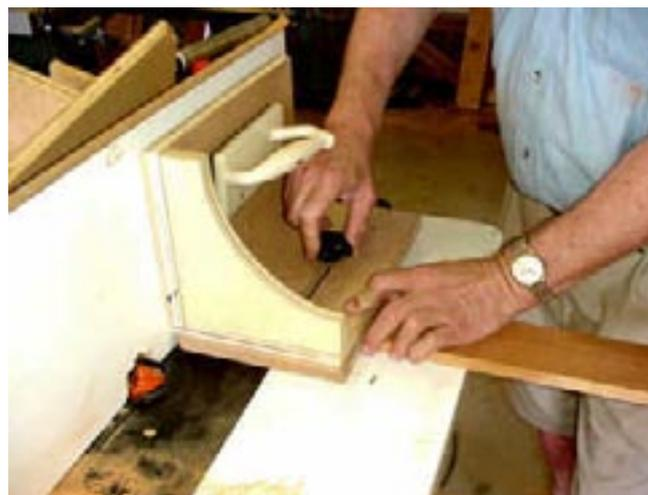
With both pieces cut, I mate them end-to-end. If the router height is exact, the seam between the two will be smooth. If "B" is low, raise the bit.
