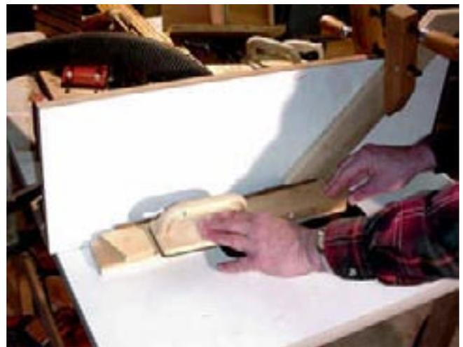
The 4 pieces fit together very well. By dry fitting them, you can see if there is any adjustment that needs to be made before glue up.
