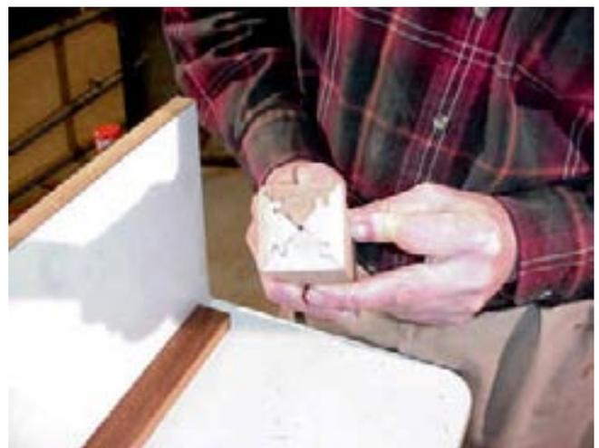
I also found that if you assemble them in order, the last joint is difficult to bring together. A better way is to assemble two sets of two sections...and then put those together to make the completed leg.
