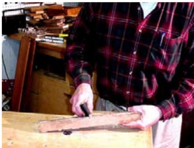
I use a rounding over plane to shape the four corners just slightly. Notice the slight gap at the far right. That is the result of the sniping at the end of the cut. I planned to trim that but found that it really was still quite tight, even with the small gap.
