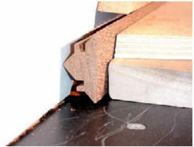
My answer to the problem is two part: 1) I made a simple push-stick that would fit the entire length of the stock and would bear pressure on the vertical mid-point. The end of the push-stick has a cut-out to grab the end of the stock...giving me better feed control.
