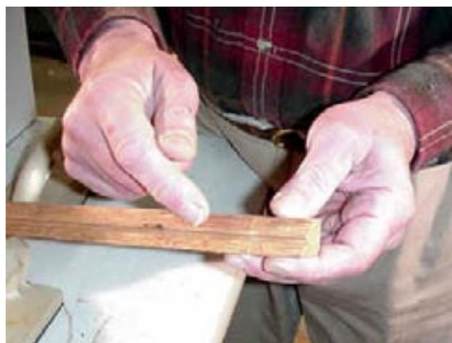
The second edge of each piece will be routed flat against the fence. While at the beginning, there is enough flat surface for the piece to be steady, at the end of the cut, the stock is only resting on the cut apex and can easily swivel away from vertical.
