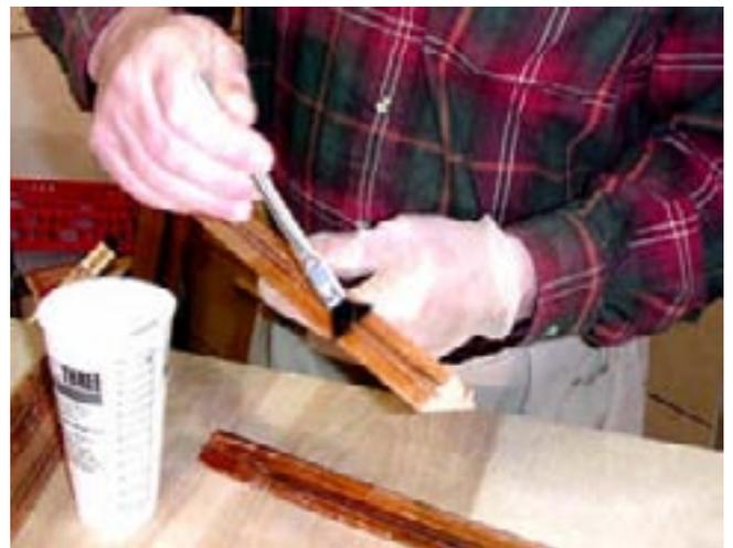
When the two pairs of sections are glued, I then apply glue to them and position them together.
