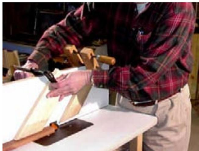
I use two rubber soled push blocks to guide the stock through the cutters.
