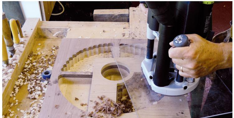
Secure the blank to your bench. With the plunge mechanism set at the top of its travel, place the router over an open area on the template. Make sure the cutter is not contacting the wood and turn on the router. Gently slide the router to the template edge and begin your cut. Continue the cut around the opening.
