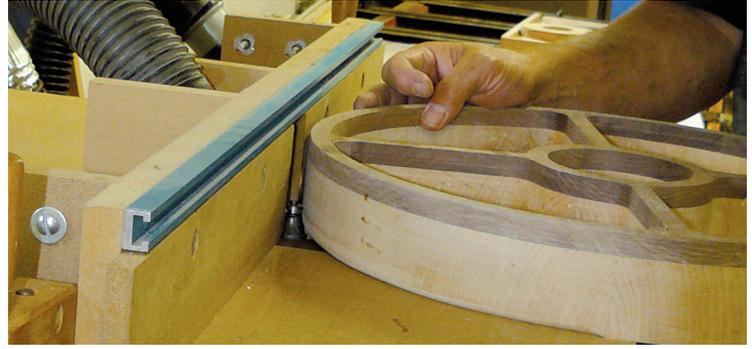
With the bowl sanded round and the band saw marks removed, head to the router table for some final shaping. Mount a 12,7mm roundover bit in the router and round over the bottom edge of the bowl.
