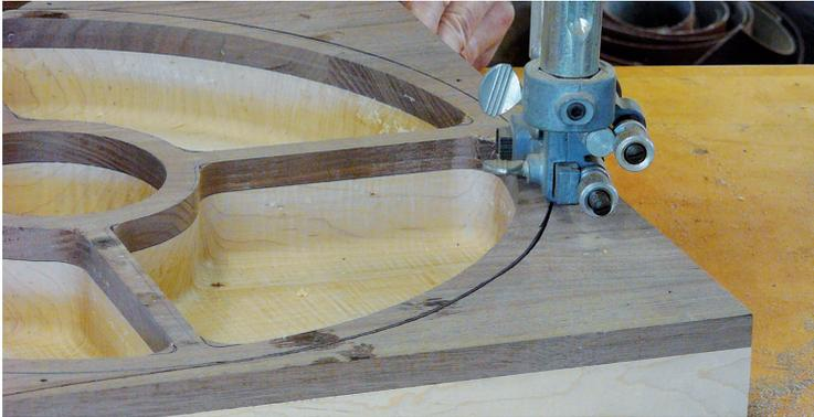
Take the blank to the bandsaw and cut off the excess stock. Take care to cut up to the layout line. Go slowly and do your best to make the cut smooth and accurate. It'll save you a lot of sanding later.
