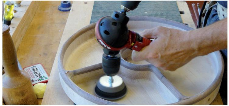
Sand the interior of the bowl using a soft disc. These discs are commonly used by lathe turners on lathe-turned bowl interiors. Start with 80-grit and work your way up to 220-grit. Finish sanding the outside with an orbital sander. Now you're ready to apply a finish. A great food safe finish for wood is walnut oil. You'll find it at most health food stores. It dries hard and is totally non-toxic. Other food safe finishes include mineral oil, salad bowl finish and shellac.
