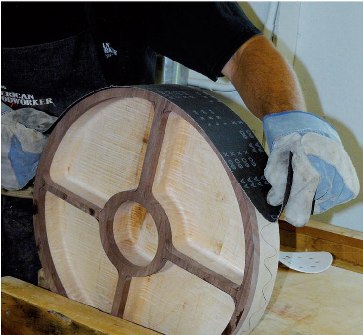
The bowl will come off the band saw round but rough. Sand the band sawn edge smooth and fair. A good way to sand the edge on a round bowl is to use a sanding belt. Pencil marks on the outside edge tell you where the low spots are and where you've sanded. Clamp the bowl blank in a vise (use scrap wood to protect the bowl from iron jaws) and sand the edge like a shoeshine polishes a shoe.
